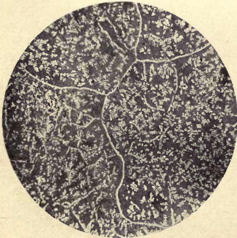
Fig. 35a. \times 40 Alloy 48. Cu 66.0 Slowly cooled in Sn 17.0 furnace. Zn 17.0. \gamma + eutectoid.
